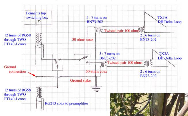
The double FT140-J chokes should provide at least 3.000 ohms impedance, more than enough for common mode blocking on 160 meters. "J" material is the same as "75" with high resistive characteristics.
