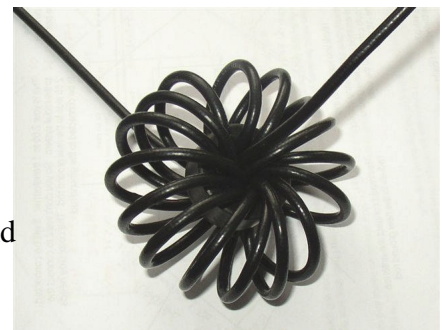
RF choke: 16 turns of RG58 on FT140-J
