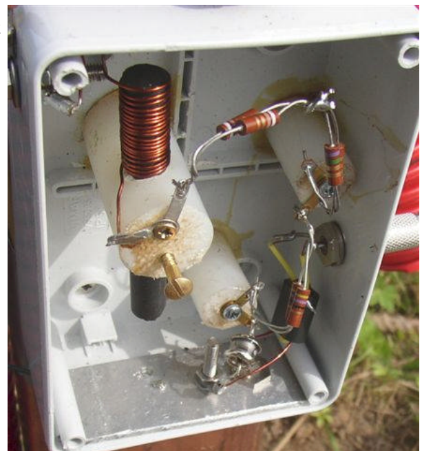
A matching box completed and tuned
