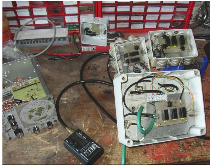
On bench test with the RF1 analyzer
