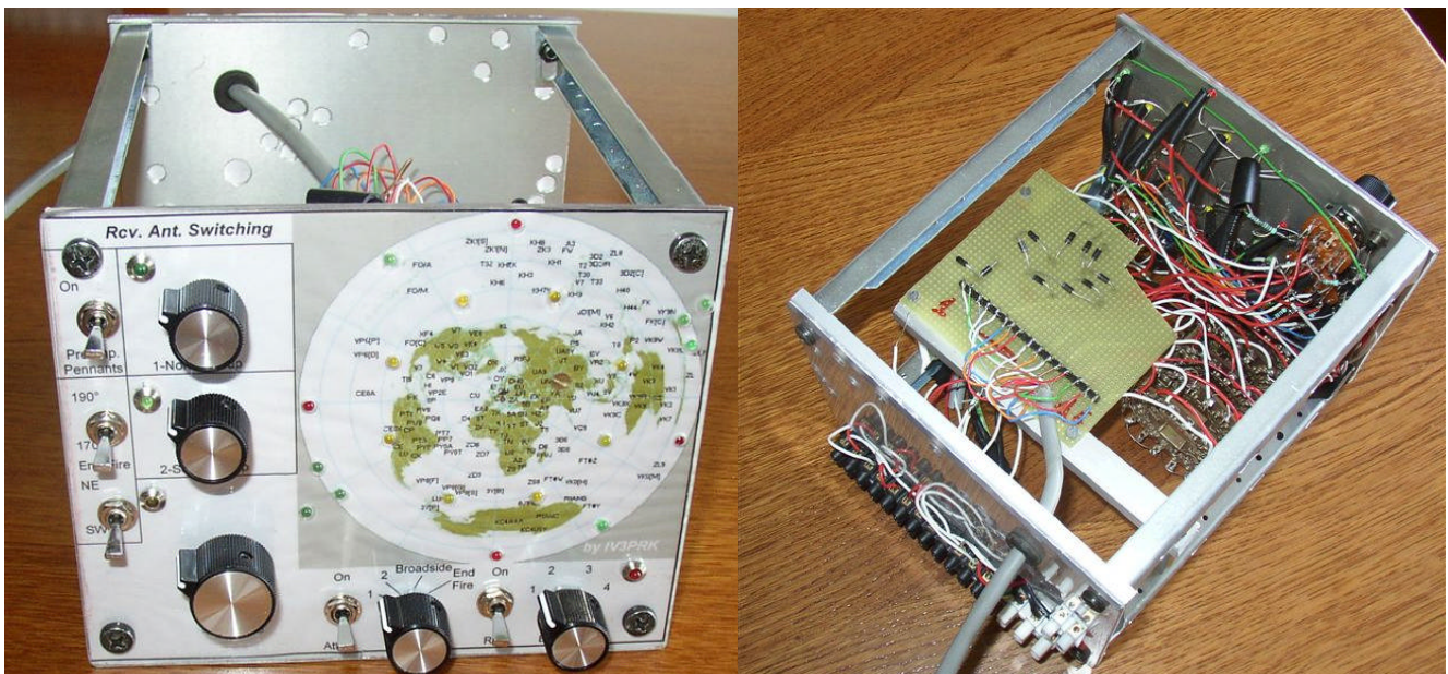
The new receiving antennas control box. The big rotary switch in the right picture is used for the 4-square array
