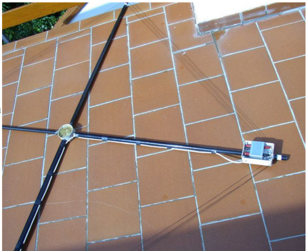
The Hi-z amplifier aluminium box with banana plugs in a sealed electrical plastic box
