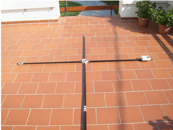
One meter sections of one and half fiberglass fishing rods with a crossing joint through a round electrical derivation box reinforced by means of polyester resin
